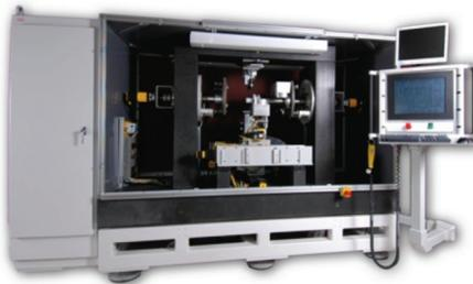
*Figure: A custom-designed automated machine for rapid fiber optic coil winding for strategic, navigation, and tactical grade gyroscopes.
