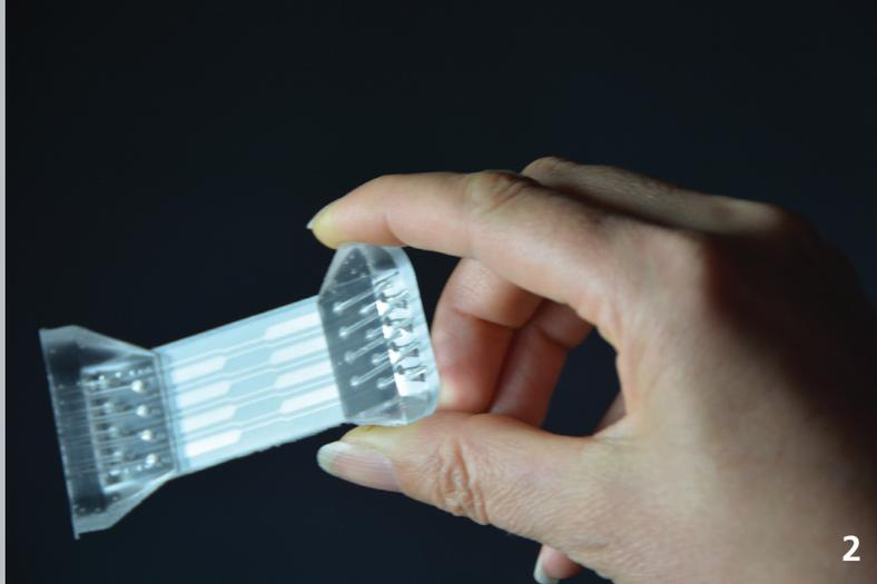
Fluorescence is monitored in real-time for the quantitative detection of pathogens at concentrations as low as 10 DNA copies per microliter. (Fernández-Carballo et al. *Biomed. Microdevices* 2016, 18, 34).
